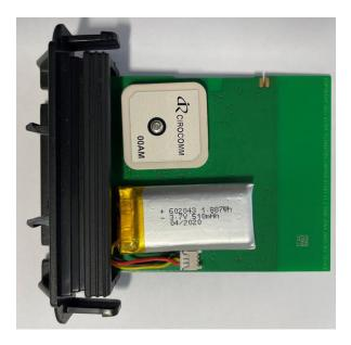
Do not attempt to remove the battery from the cover, once it has been stuck down, as prising or bending could lead to explosion/fire and smoke.
