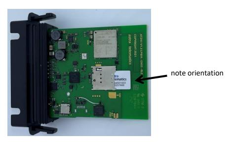
Note that the AT242 powers up when the SIM is fitted
