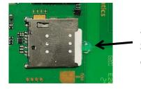
a drop of hot glue can be applied to prevent movement of the SIM, in applications where vibration may cause inadvertent SIM extraction
